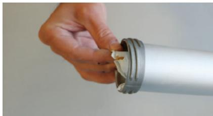
7 Make sure the entire Skamol Glue bag is inside the Skamol Glue Pistol.
