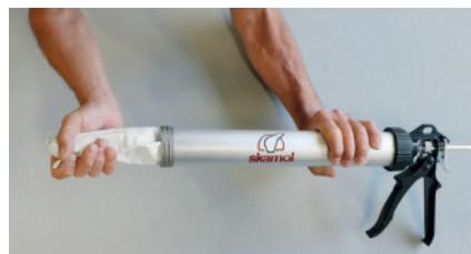
5 Insert the Skamol Glue bag in the Skamol Glue Pistol. The small hole must point towards the opening.
