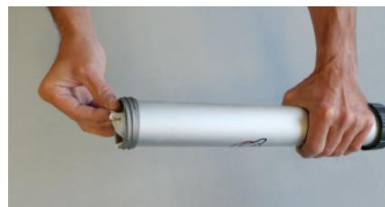
6 Twist the Skamol Glue bag to fit it easily in the Skamol Glue Pistol.
